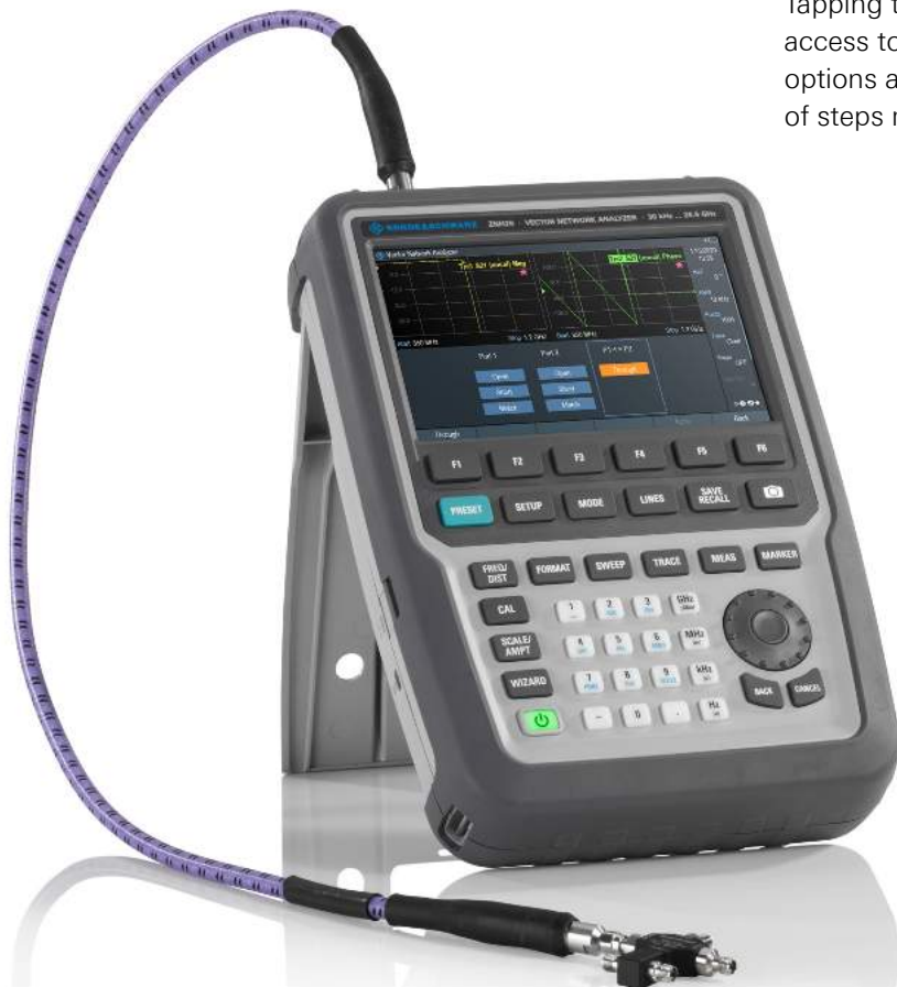
The R&S®ZNH enables flexible, user-defined calibration sequences.
