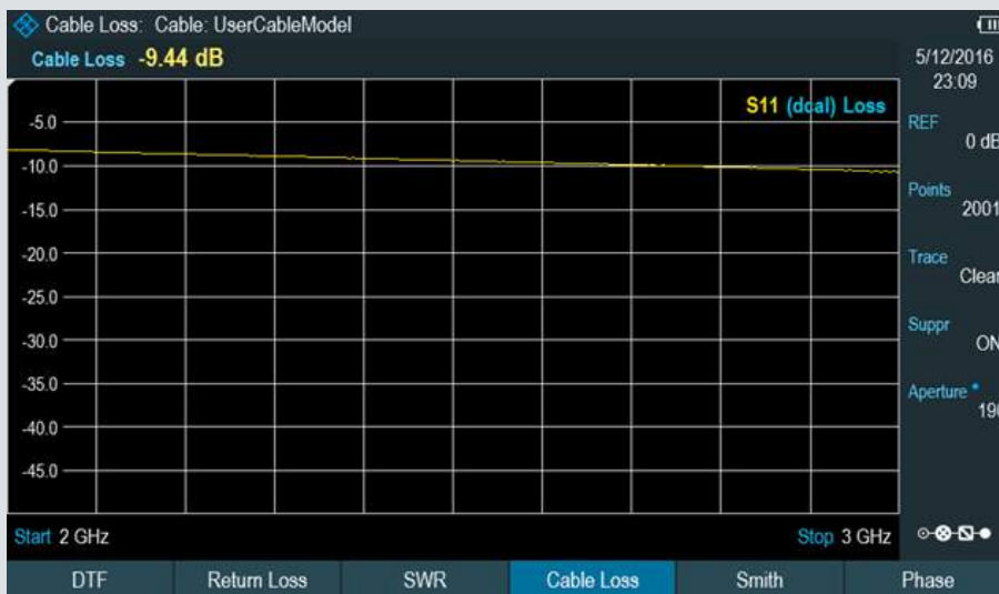
One-port cable loss measurement
