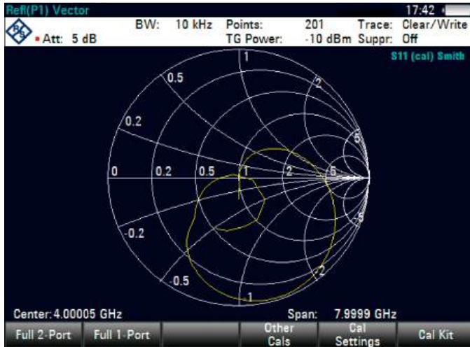
Vector network analysis: measurement with Smith chart
