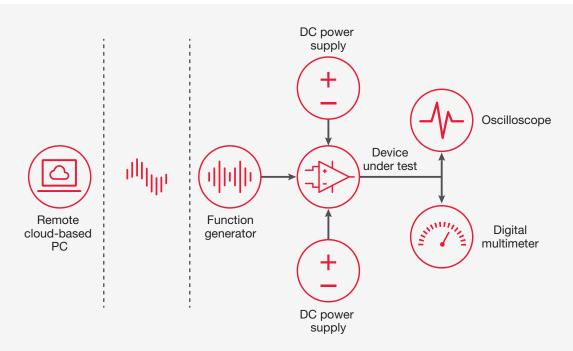
Figure 1. Smart Bench Essential Series instruments work together to test the DUT
